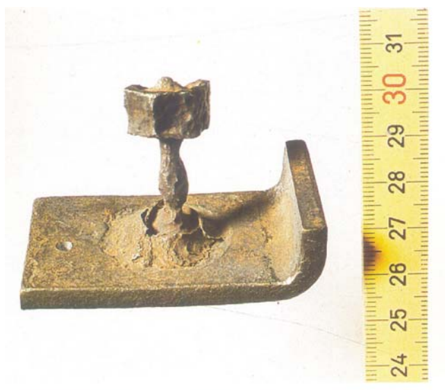
Figure 3.1 Galvanic corrosion attack of carbon steel bolt in contact with 12% Cr steel (AISI 410) stainless steel plate in hydrocarbons contaminated with traces of salts. This is ray lamp of a distillation column. (Source: During (1988). Reproduced with permission of Elsevier.).
