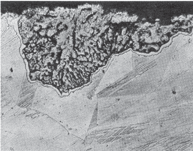
Figure 3.11 Etched cross-section through dezincification plug (Source: Verink and Heidersbach (1972). Reprinted with permission from STP 516- Localised Corrosion- Cause for Metal Failure Copyright ASTM International.).
