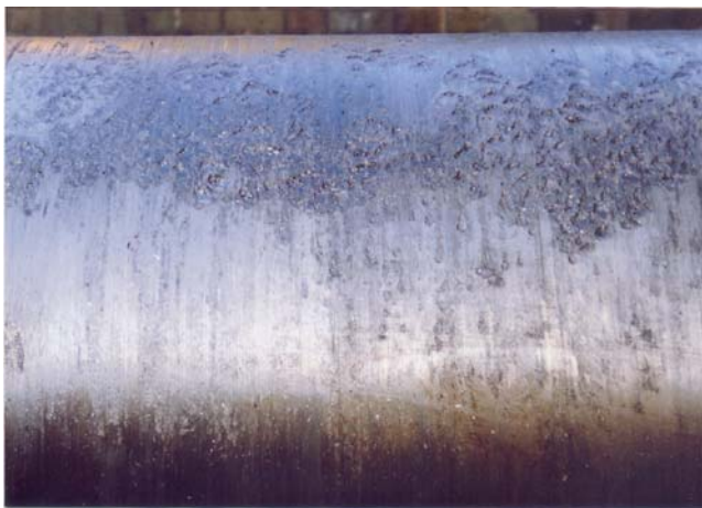
Figure 3.15 Cavitation damage appearing as bright pits on a damaged propeller shaft of a ship. The alloy is beta brass.
